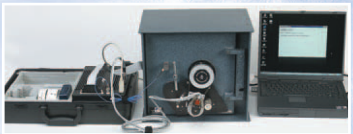
6. Connect the cables between the motor and the microphone, the SoftDrill™ and your laptop.
