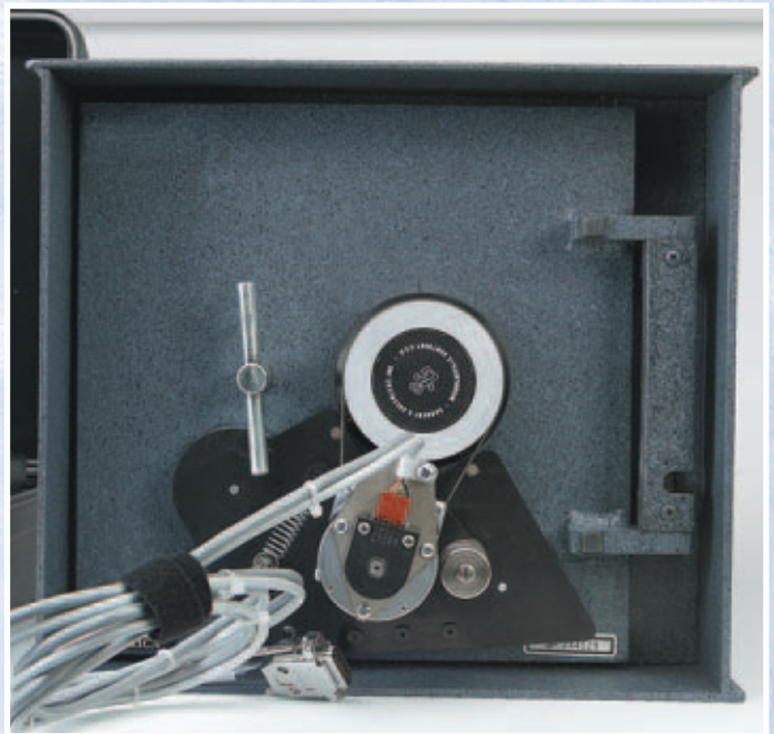
4. Attached the precision stepper motor to the mounting bracket and slip the belt over the pulley.
